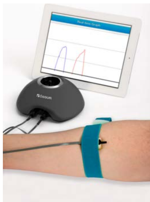
Virtu-Limb™ to measure myoelectric signals
