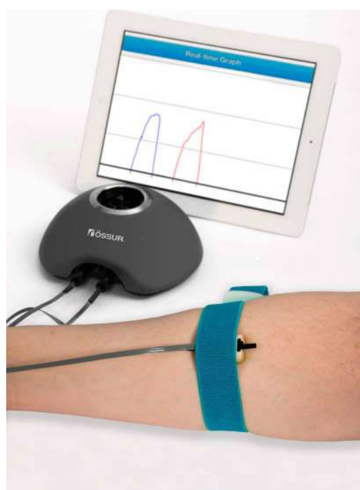
Virtu-Limb™ to measure myoelectric signals
