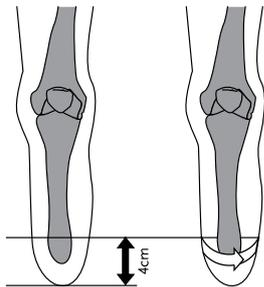
With the tissue of the residual limb hanging down, measure 4cm proximal to the distal end of the limb and mark this point on the skin. Measure the circumference of the limb at this point with medium tension on the tape measure.
