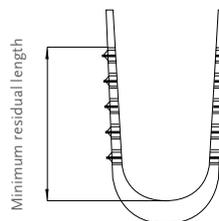
Matrix size varies depending on the liner size, the smaller the liner the shorter the matrix.
