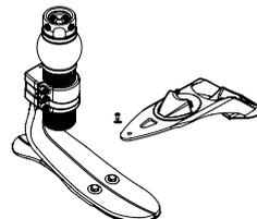
Caution: Due to restricted space with the Re-Flex Shock shock module and Unity, SSPE\* kits allow for only 2 full turns of downwards adjustment from the tallest setting. Re-Flex Rotate modules can be set to any height within their designed limits.
