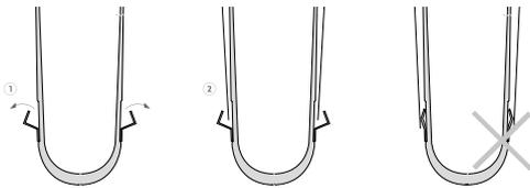
Note: Loss of suspension will occur if a sock is placed over the HSM Seal.
