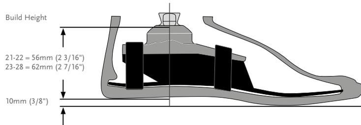
Note. Flex-Foot Balance with Unity has the same build height as Flex-Foot Balance.
