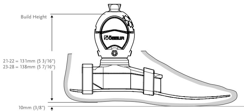
\*Note. Flex-Foot Balance with D/P Flexion with Unity has the same build height as Flex-Foot Balance with D/P Flexion.
