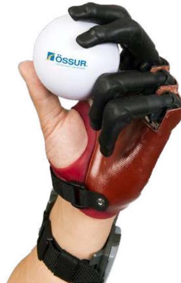
Gesture control enables an automated grip to be accessed by moving the i-Digits Quantum in one of four directions.
