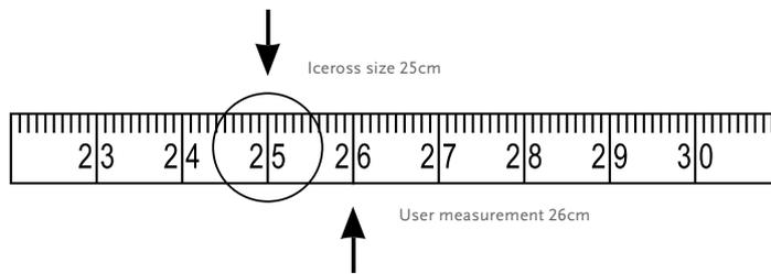
The measurement taken corresponds to the size of Iceross to be used. Select the liner size matching your measurement or, if between sizes, select the next size below. Do not select a size larger than your measurement or more than one size below the measurement. E.g. if the circumference of the limb measures 26cm, select Iceross size 25.
