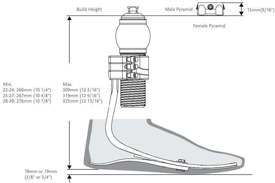
\*Note: Re-Flex Rotate with Unity has the same build height as Re-Flex Rotate.
