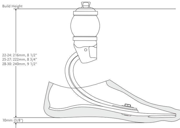
\*Note: Pro-Flex XC Torsion with Unity has the same build height as Pro-Flex XC Torsion.
