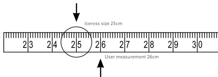
The measurement taken corresponds to the size of Iceross to be used. Select the liner size matching your measurement or, if between sizes, select the next size below. Do not select a size larger than your measurement or more than one size below it. E.g. if the circumference of the limb measures 26cm, select Iceross size 25.
