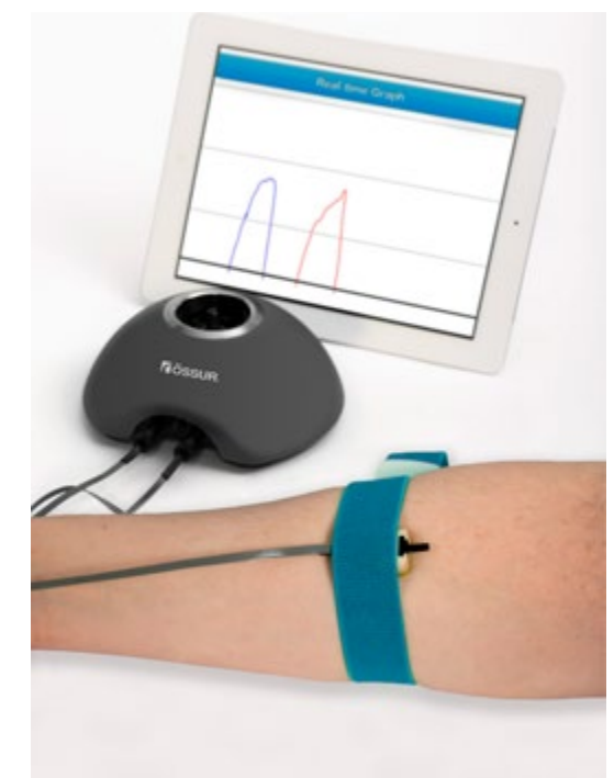
Virtu-Limb™ to measure myoelectric signals
