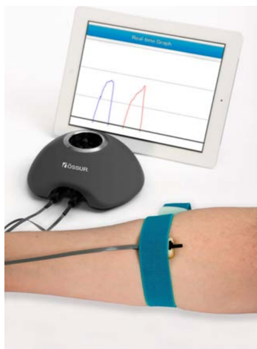
Virtu-Limb to measure myoelectric signals
