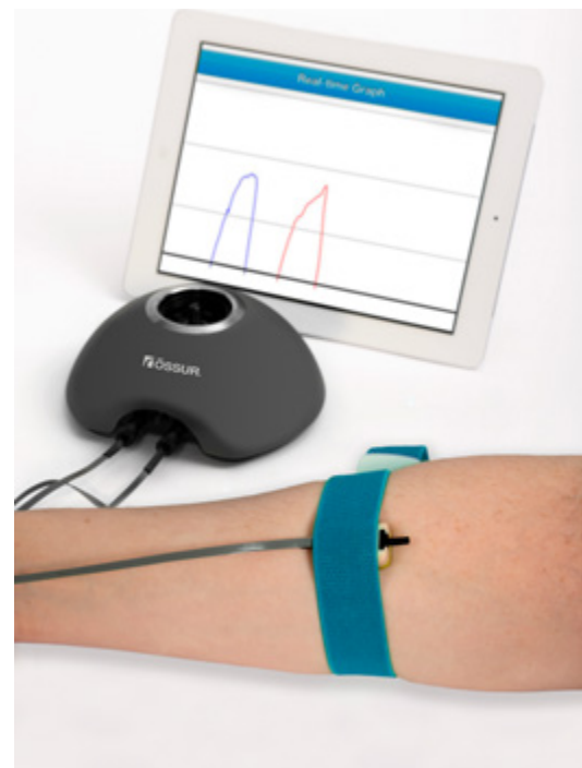
Virtu-Limb™ to measure myoelectric signals
