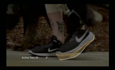
**Active Dorsiflexion** means that with every step the powered ankle raises the toe to increase toe clearance and repositions it for heel contact, in perfect sync with the wearers gait profile.
