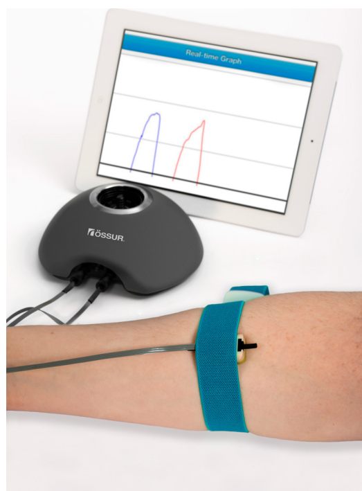
Virtu-Limb to measure myoelectric signals
