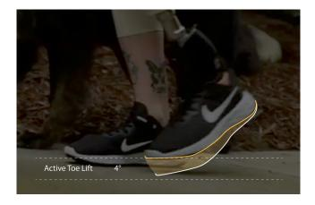
**Active Dorsiflexion** means that with every step the powered ankle raises the toe to increase toe clearance and repositions it for heel contact, in perfect sync with the wearers gait profile.
