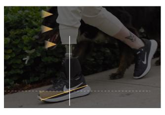
**Terrain Adaptation** provides real-time adaptive ankle function with sensors that continually monitor the surface angle and acceleration to pre-position the foot for inclines, declines, and stair ascent and descent.
