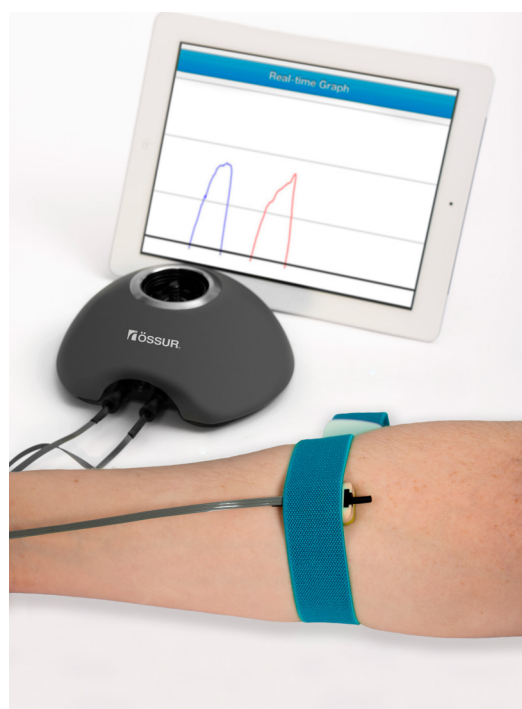
Virtu-Limb to measure myoelectric signals
